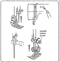
NOTE: Raise the needle bar to its highest position by pressing the Up/Down Needle Position Button:
